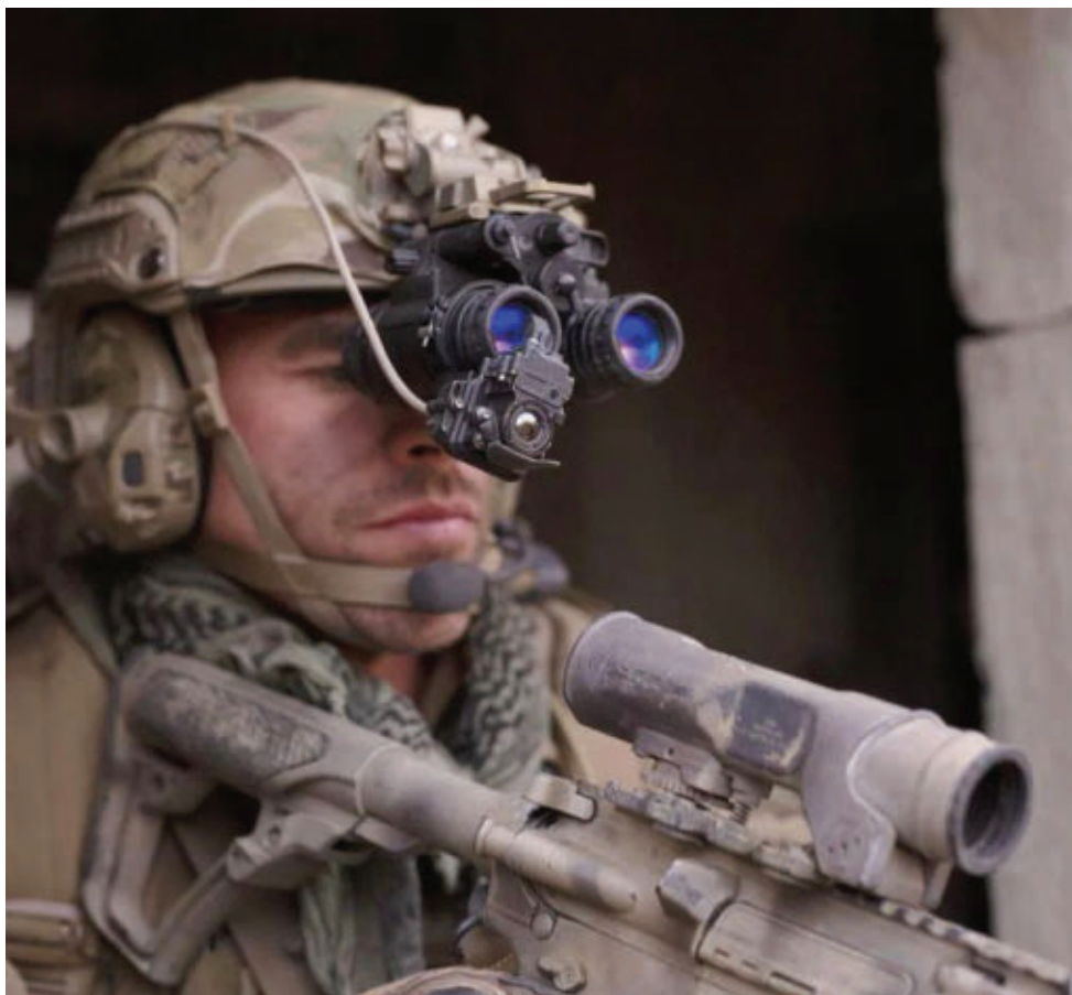
▲ The lightweight SBNVG enhances Marines depth perception, and combines longwave infrared with light-amplification sensors.
