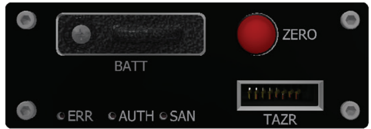
▲ Crystal Group developed the Tamper and Zeroization Response (TAZR) device that monitors bus signals, tamper sensors, and remote commands to eliminate the threat of compromised data.
