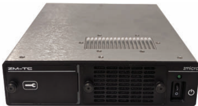
▲ ZMicro offers a distributed computing approach to enable use of thin-clients for edge computing applications, with a 3.2-pound computer that sends data back to a central server.
